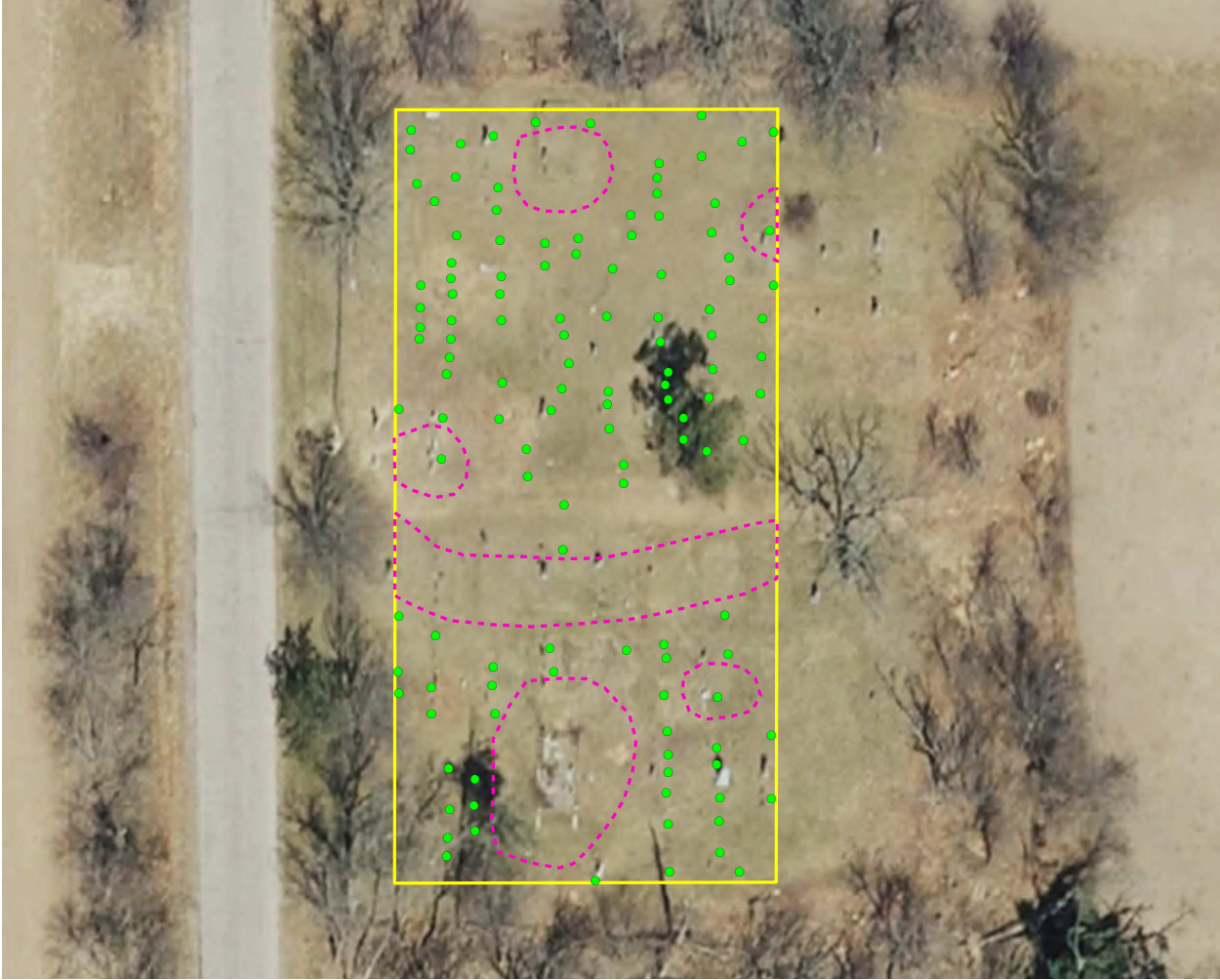
Figure 9: Geomagnetic anomalies superimposed on an aerial image of Morrill Cemetery. The purple dashed lines mark areas where the geomagnetic field of subsurface deposits made it difficult to identify more subtle anomalies.
