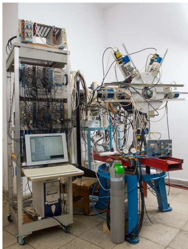
Fig. 2 The Atomki 5 arms spectrometer used in the first {}^8\text{Be} measurement in 2016
