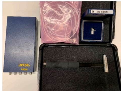
Figure 5. Impact hammer, accelerometer, and the acquisition device with DATs software.
