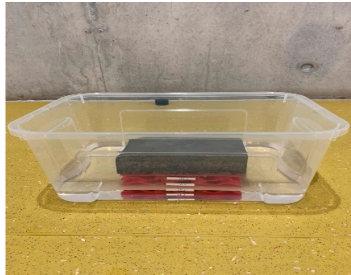
Figure 9. Porous bridge bearing at a flood level.
