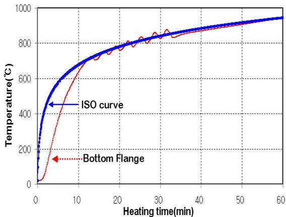
Figure 3. Temperature-time curves compared
