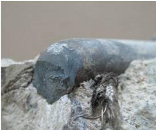
(b) Failure of headed stud
