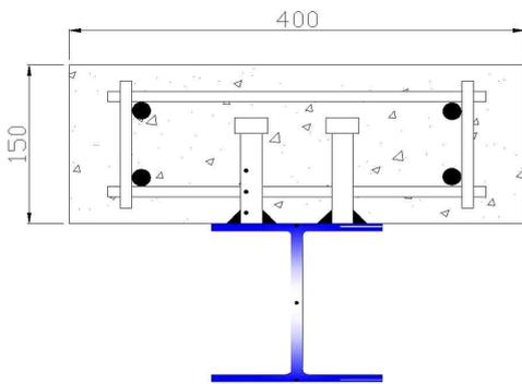
(a) Composite beam with ribbed bar
