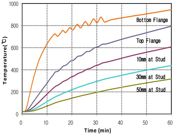
Figure 7. Temperature-time curves in steel and stud connector of 60 minute specimen number 2.
