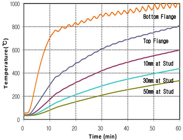
Figure 6. Temperature-time curves in steel and stud connector of 60 minute specimen
