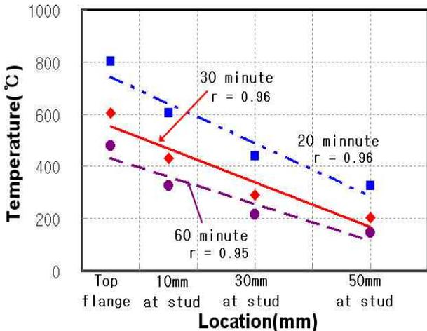
Figure 10. Average temperature-thermocouples location in top flange and stud connectors.
