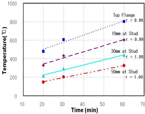
Figure 9. Average temperature-time curves of top flange and stud connectors in furnace.
