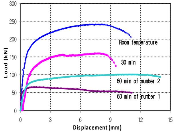
Figure 4. Load-displacement curves for push out test.
