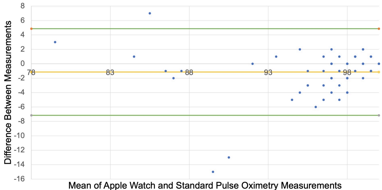
Fig 2. Bland Altman Analysis of AW6 pulse oximetry compared to standard. Horizontal lines represent the mean difference of oxygen saturation between the Apple Watch 6 and standard pulse oximetry and the upper and lower limits of agreement (LOA). Upper and lower LOA represent +1.96 and -1.96 standard deviations respectively. Points may represent multiple patients.
