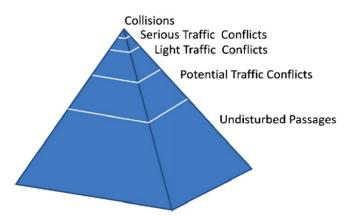
Figure 3. Pyramid Representation of Traffic Interaction Frequency
