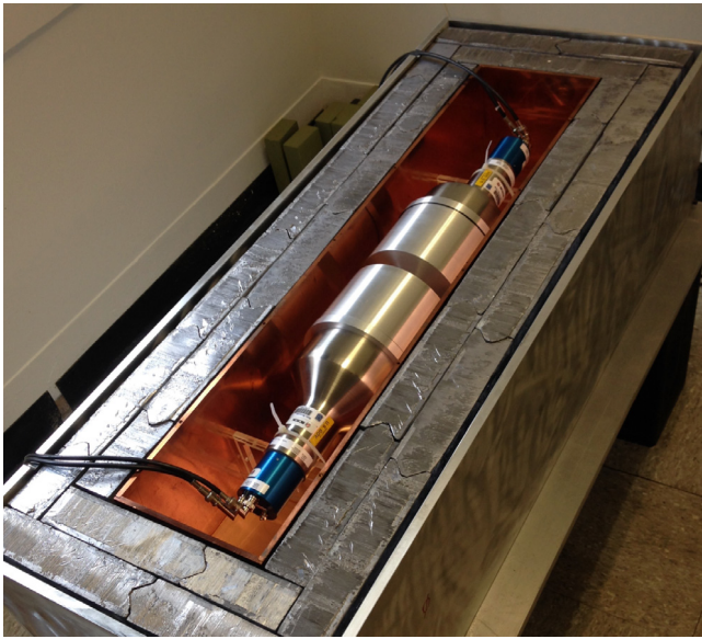
Fig. 1. (Color online) The \gamma\gamma -coincidence spectrometer consisted of two NaI(Tl) detectors inside a passive shield. The top shield, made of steel and lead, was removed to show the detector geometry.
