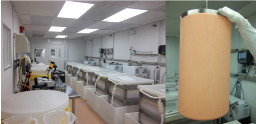
Figure 2. On the left is a view of the electroforming facility with 7 of the 10 baths visible in the photograph. On the right is a mandrel that has been lifted out of its bath for an initial inspection of the copper growth.
