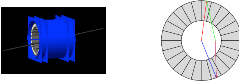
Figure 6. Left: Rotated source holder inside APEX array using Geant4. Right: Example of an event which flips sign when the source holder is translated.
