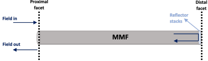
Figure 2. Single-ended optical fibre system
