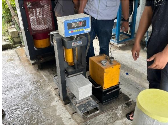
Test menggunakan flexural machine di batching plant
