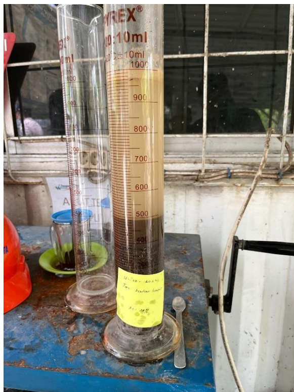
Gambar 2.11 Test kadar lumpur pada pasir di Batching Plant WBP
