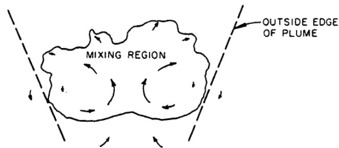
Fig. 2.12 Cross section of mean velocity distribution in a bent-over plume (Briggs, 1969).
