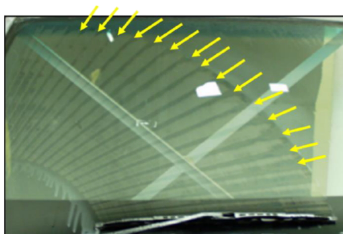
Fig. 1.4 Unwiped water caused by chatter vibration
