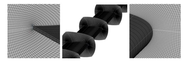
Figure 1. 7. Details of mesh refinement around direct blade modeling.
