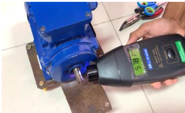
Figure 6. Rotor speed measurement using a tachometer
