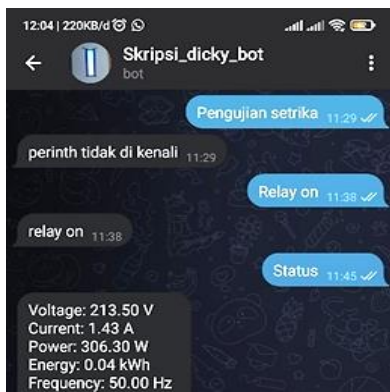
Figure 14. Power monitoring test at iron load
