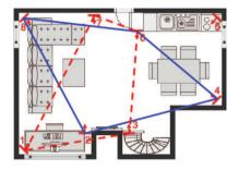
Figure 6: Microphone positions for completion models and ASC models for Situation 1.
