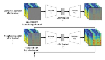
Figure 3: Block diagram of the proposed missing data completion method using an autoencoder. Only the missing channel is replaced. Normal channels are not changed.
