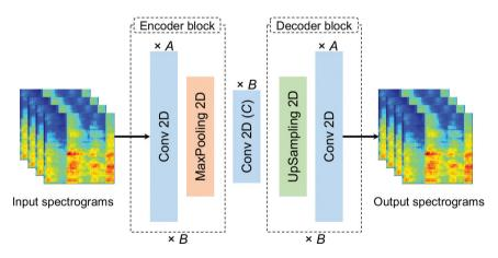
Figure 4: Network structure of the CAE used in the proposed method.
