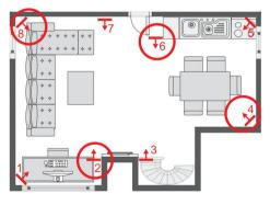
Figure 5: Two-dimensional floorplan of combined kitchen and living room [8] with selected microphone array numbers in SINS database.
