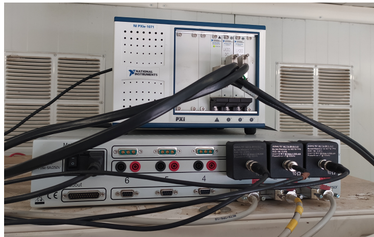
Figure 2. Part of the measurement system: NI Chassis and MCTS II.
