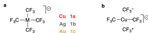
Scheme 1. Homoleptic coinage metal(III) trifluoromethyl compounds (a) and bonding scheme suggested by Snyder for the copper derivative (b). [10]
