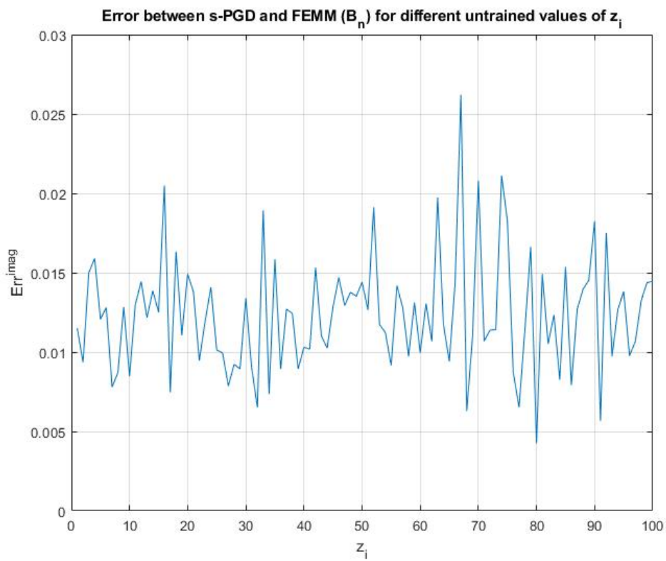
Figure 4.26 – Relative error of the s -PGD model (nonlinear B-H relationship) to determine the imaginary part of B_n for different untrained z_i . Error criteria of Eq. (4.26) is used.
