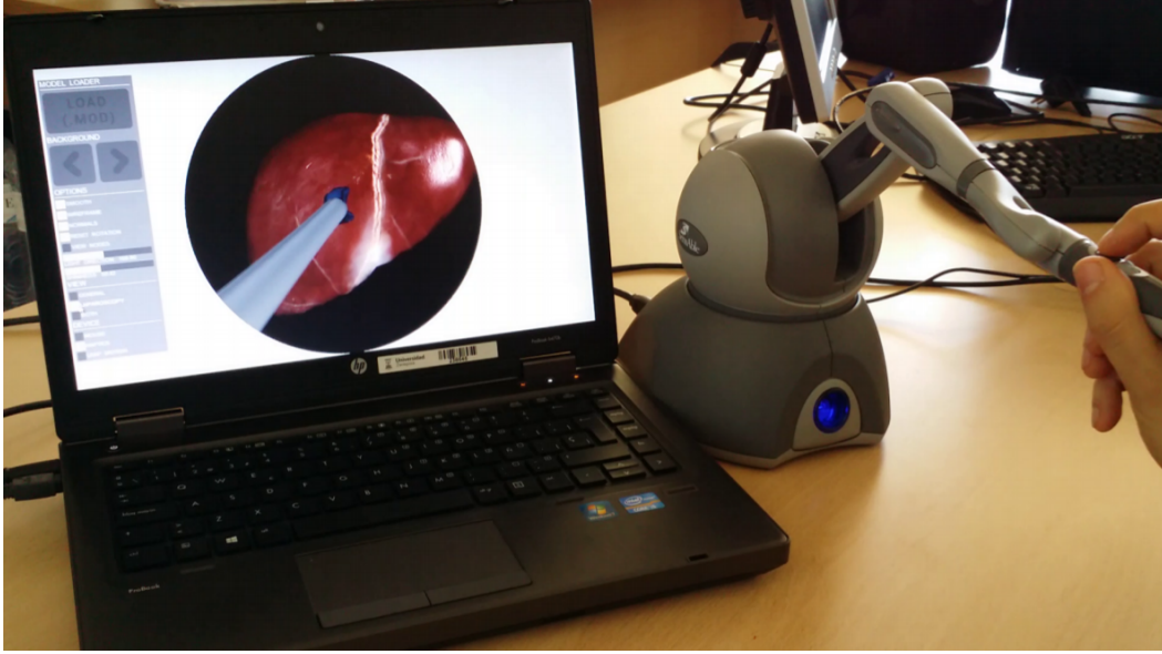
Figure 3 – Image of the haptic simulator developed with the PGD methodology. This simulator is able to provide the solution of a complex nonlinear mechanic problem one thousand times per second. Special thanks to the Applied Mechanics and Bioengineering group of the University of Zaragoza (specifically, Professor Elias Cueto) which authorised the diffusion of the image in the present thesis.
