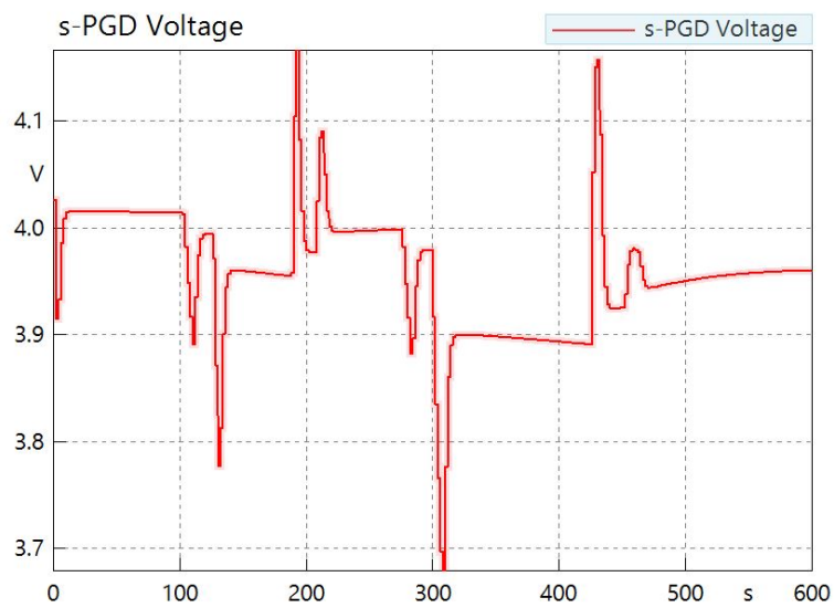
Figure 7.26 – Cell voltage predicted by the s -PGD model during the simulated itinerary.
