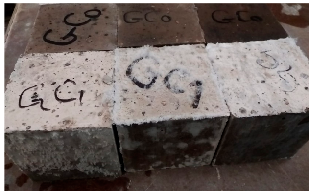
Figure 5. Appearance of efflorescence on the surface of geopolymer concrete specimens with higher alkaline content.
