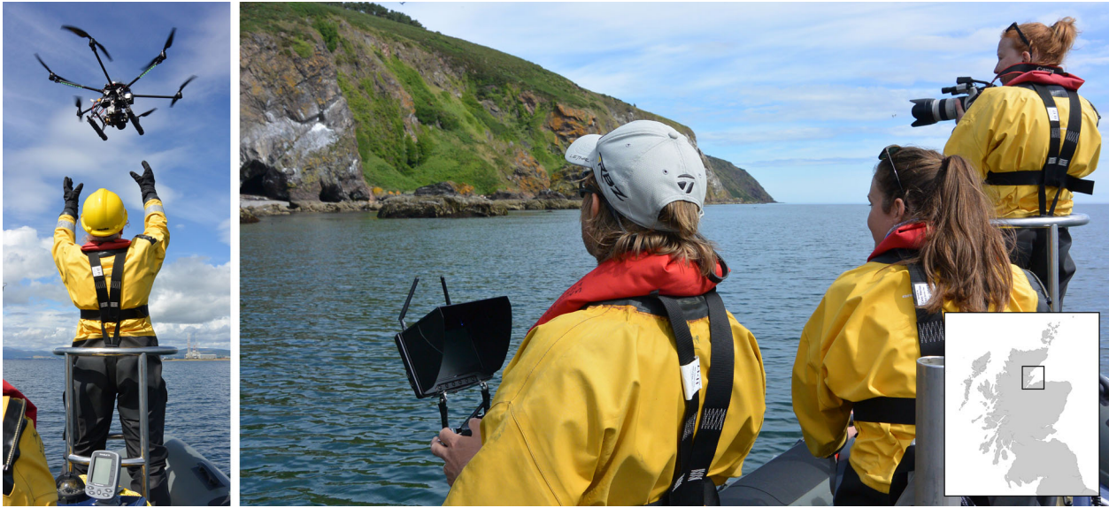
Figure 1. UAS photogrammetry surveys from a small RIB using a LexHex-44 hexacopter, including manual hand launch and recovery, operation ~30 m above a group of bottlenose dolphins with first-person view screen for the operator and concurrent photo-identification and laser photogrammetry. Inset map of the study area, the Moray Firth Special Area of Conservation, Scotland. UAS, unoccupied aerial system.
