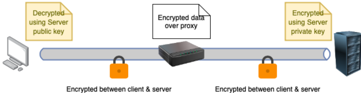
Figure 3: Visualisation of a proxy without TLS resigning. The proxy cannot decipher data sent between the client and server, as the encryption keys are unknown.
