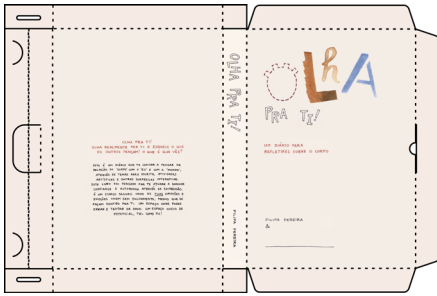
Fig. 10: Illustrated box template, 550x363mm, outside cover, to be printed in off-white 400g/m 2 paper (temporary image).
