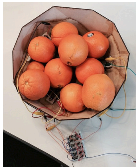
Figure 3 MDF prototype for iterating the electronics, actuators, and movement of the bowl while bearing weight.
