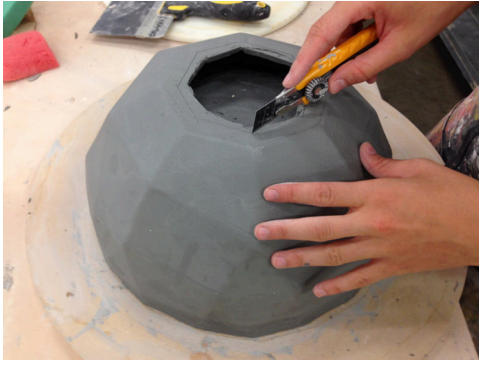
Figure 9 Trimming the opening of the bottom of the bowl after the form has dried.
