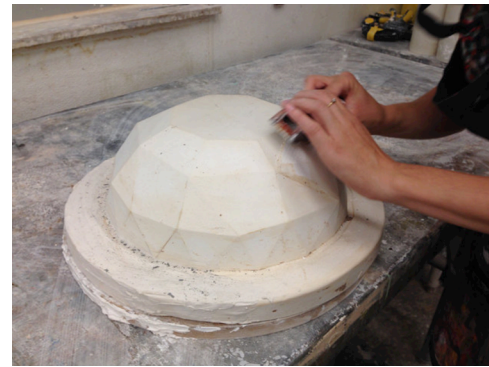
Figure 8 The plaster mould being manually “fixed” to sharpen the angles to recover fidelity of the CAD model and laser cut prototype.
