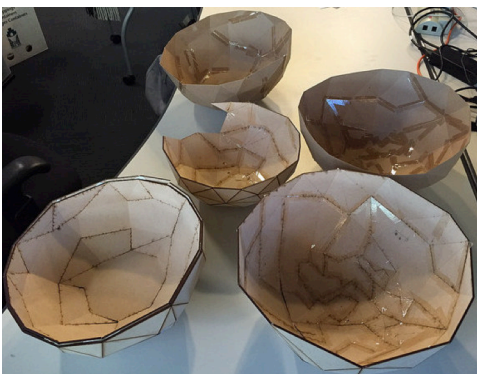
Figure 2 Examples of some of the many alternative forms produced with 123D Make in cardboard and MDF.
