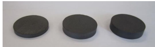
Figure 3.8. Ballard’s graphite BPP samples with different nominal thicknesses of 2.95, 4.94 and 5.84 mm
