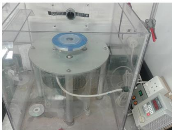
Figure 2-9: The image of the rotating platform used for spinning the CD-NBA chip.
