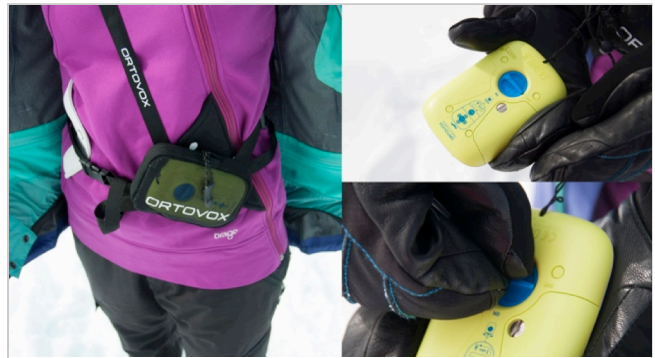
Figure 3. The beacon is worn on the torso in a harness. Some functions and buttons are challenging to use with gloves.
