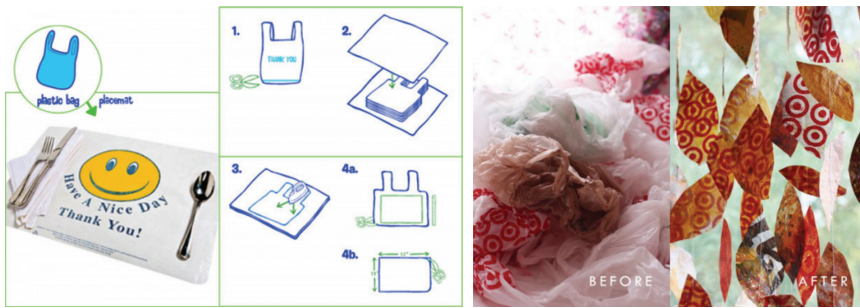
Fig. 4. (a) Flow diagram to make fused plastic bag fabric by Tiffany Threadgould and (b) plastic leaf garland 11 by “Aunt Peaches”.
