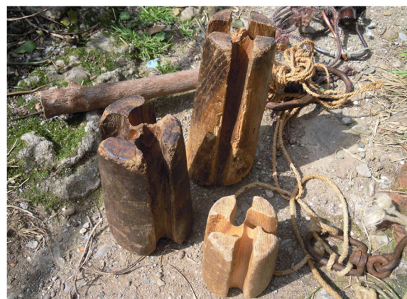
Figure 6 Tools made of Castanea sativa wood (the two bigger ones). These tools are used to twist the single threads for weaving ropes.
