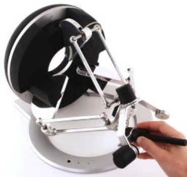
Figure 5: Delta 6 device by Force Dimension
