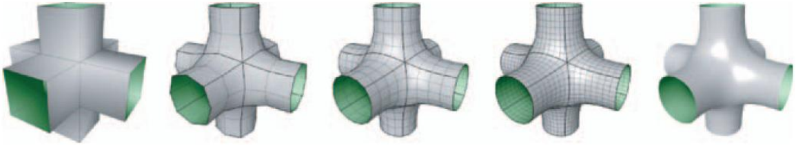
Figure 2.11: Refinement based remeshing. Starting from a base mesh on the left, the mesh is iteratively refined to the final smooth mesh on the left. The figure is taken from [3].
