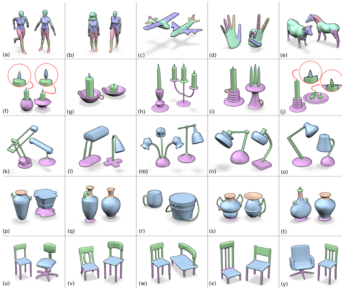
Figure 3.5: Part correspondence results via joint labeling. Aside from the failure cases in (j), (t), and (y), our method succeeds even under significant geometric and topological variations between the matched parts, while purely content-driven methods would fail (see Figure 3.7 for a comparison). Corresponding segments between a pair of shapes are shown with the same color.
