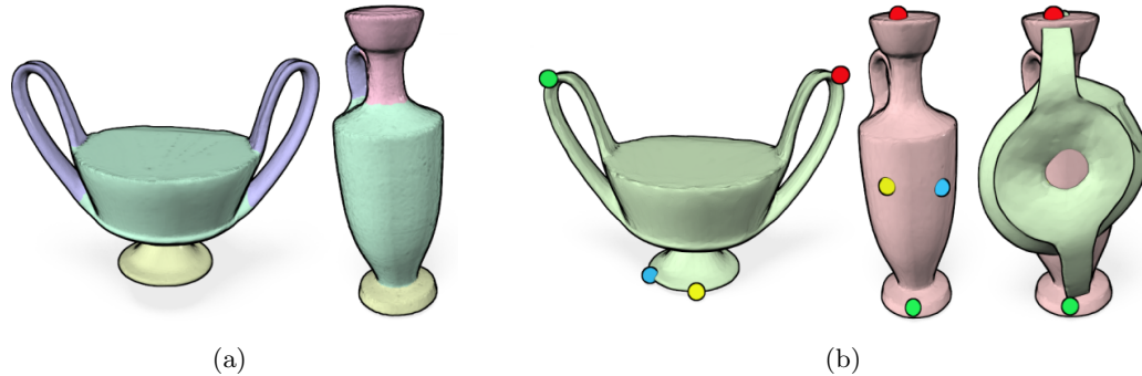
Figure 1.1: Correspondence between dissimilar man-made shapes. (a) A meaningful correspondence between shape parts is shown, where corresponding parts are implied by matching colors. Note the significant geometric and topological differences between the two shapes. The correspondence was obtained with our supervised knowledge-driven approach. (b) A feature-to-feature correspondence, where the matched feature points are shown with corresponding colors. The implied alignment is shown to the far right. This result was obtained with a state-of-the-art feature matching method (the deformation-driven method of Zhang et al. [2008]), which is not able to handle such a challenging case of dissimilar shapes.
