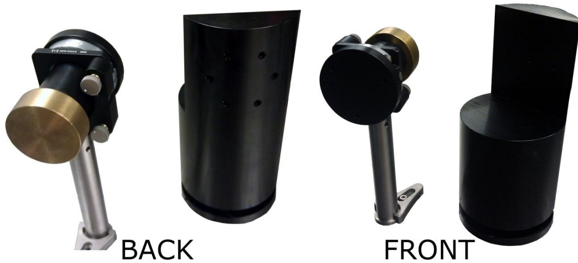
Figure 31 – Back and front views of old (left) and new (right) mounts (same scale).
