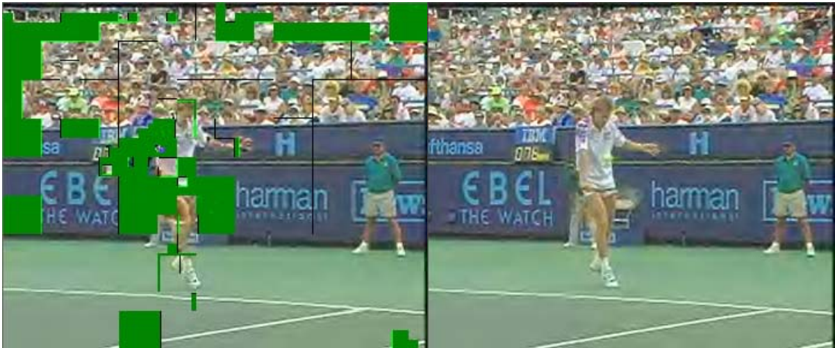
Figure 3.2: Frame that is reconstructed by Motion Concatenation only (left) and the coded loss-free frame (right)
