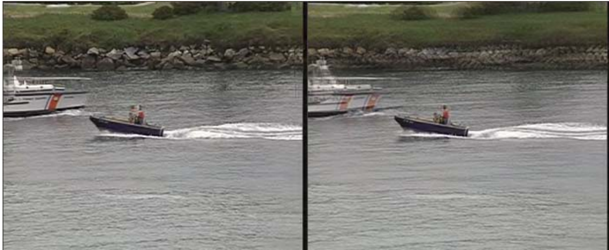
Figure 4.5: Frame that is reconstructed by complete error concealment (left) and by zero-motion error concealment (right) in two-level MCTF
