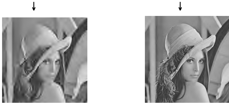
Figure 2.1: Decoding the embedded bit stream produced by SPIHT: the more bits are decoded, the better the resulting image quality
