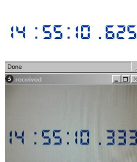
Figure 2.6: Part of the captured screen showing the local clock at the receiver (top), and the received image of the transmitter's clock (bottom), with millisecond precision
