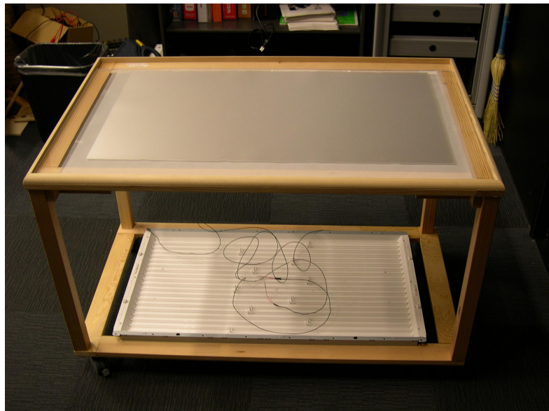
Figure 40: The backlight separated and reintegrated into the table structure.
