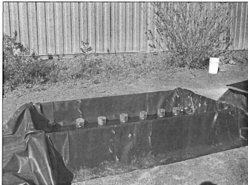
Figure 3.4 Experimental set-up of outdoor incubators used in all photobleaching experiments. One-litre microcosms were placed either a) under different UV filters held in place using wooden frames and rope or b) in an open incubator. Incubators were placed in an area of the Inuvik Research Centre grounds that was in direct sunlight between 9:00 AM and 9:00 PM, MDT.
