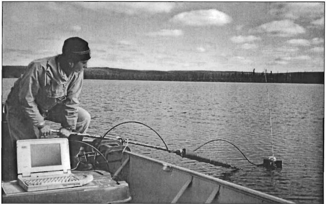
Figure 2.6 The OL 754 portable high accuracy submersible UV-VIS scanning spectroradiometer (Optronics Laboratories), configured for field scans. The submersible integrating sphere and depth indicator can be seen to the right. The 3 m long parallel swing arm allowed the operator to position and hold the integrating sphere at a specific depth while a series of spectral scans were taken.
