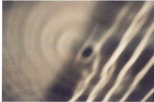
Figure 2.12: Two wooden blocks placed in a circular ripple tank with a slit between them, creating circular waves. Beneath the ripple tank was a sheet of white paper, where the wave patterns appeared due to a light source above the ripple tank. ©Armed Blowfish. Used by permission under the BSD license. 7
