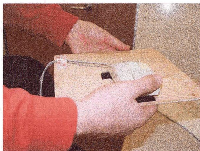
Figure 8.2: Three DOF input device for the orientation task.
