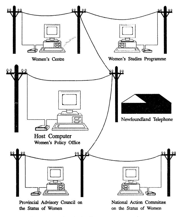
Users at different locations in a local calling area connect to a host computer through the local phone system. Once connected to the host computer, users at all locations use software on the host computer to send and receive electronic mail and upload and download files. Users outside the local calling area can make long distance calls to the host computer.
