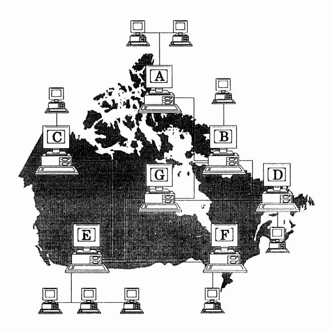
Users connect to a local node and use the electronic mail software running on their local node to send and receive messages. It is possible to send messages between most nodes. The address from one node to another reflects pathways between those nodes. To run a bundled E-mail group, one node (i.e. G) is designated as a host node. Mail from all nodes is sent to that node, bundled and redistributed. Some nodes (i.e. E and B) forward mail to other nodes.
