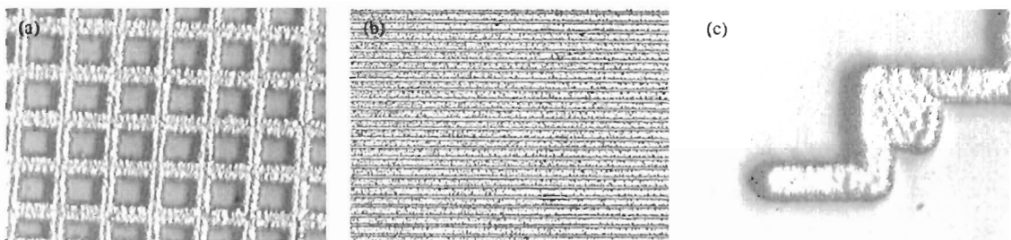
Figure 7.27 Electroplated Ni grown on patterned Bi/In resist on Si wafer. (a) Ni mesh. The spacing between two lines is 10 \mu\text{m} (50 \times optical). (b) densely plated Ni lines with 5 \mu\text{m} spacing (100 \times optical) and (c) a small pattern of 4 \mu\text{m} square with 2 \mu\text{m} wide line (800 \times optical).
