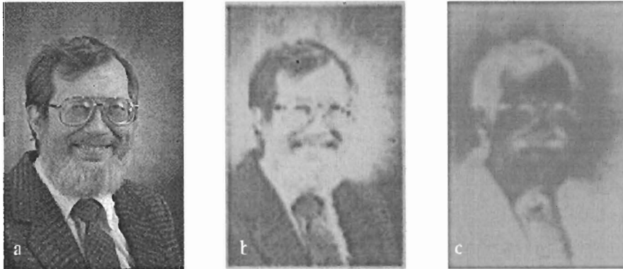
Figure 8.21 More complicated grayscale photo was successfully made on a Sn/In substrate: (a) the original 8-bit grayscale bitmap file; (b) the front-lit image of picture written on Sn/In film; and (c) the back-lit image.
