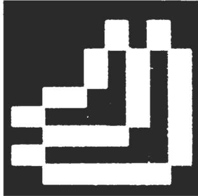
Figure 5.6 One of the patterns on the Al photomask used for the projection. The width of the rectangular lines is from 50 to 150 \mu\text{m} .
