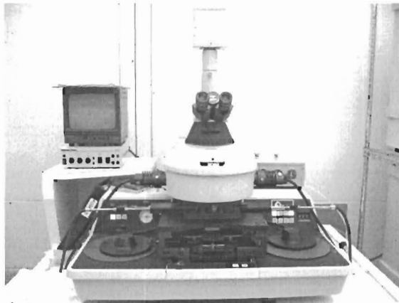
Figure 4.14 Quintel 4 inch mask aligner with a Hg arc lamp as light source is used to expose regular organic photoresists.
