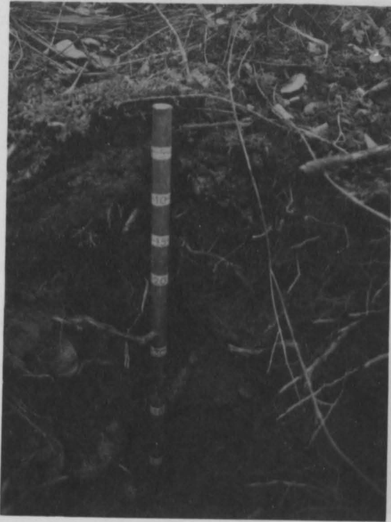
Fig. 18. The soil profile at plot 1 (control site). Note the abundance of litter and the distribution of roots throughout the profile. Rounded pebbles up to 20 cm in length were common (The measuring stick is graded in cm)
