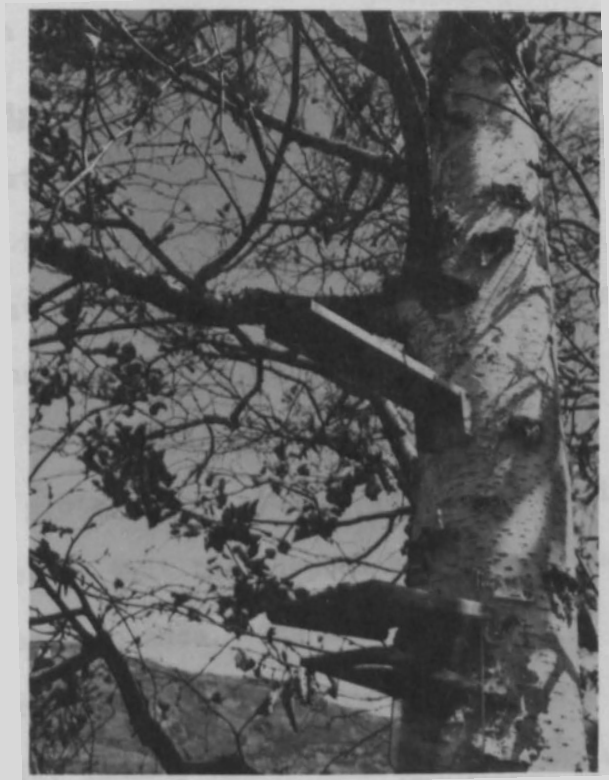
Fig. 11. The lead dioxide sulphation plates used in the estimation of current sulphur dioxide levels in the study area. The upper plate is the standard 'Huey' equipment mounted with the lead paste facing downwards; the lower plate, facing upwards, is in a modified 'Cominco' holder
