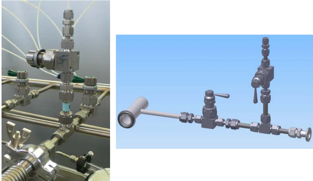
Figure 21: Photography and schematic of one extraction unit (Own source).
