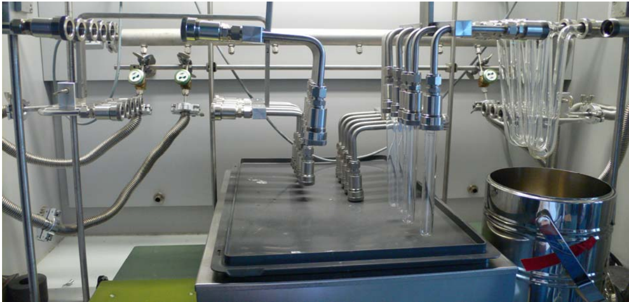
Figure 17: Photography of cryogenic vacuum extraction device for soil and plant material of the PSI (Own source).
