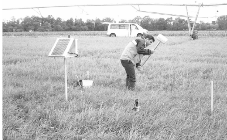
Figure 3.13: Soil sampling for irrigation scheduling and soil-specific calibration of the EnviroSCAN soil moisture sensor
