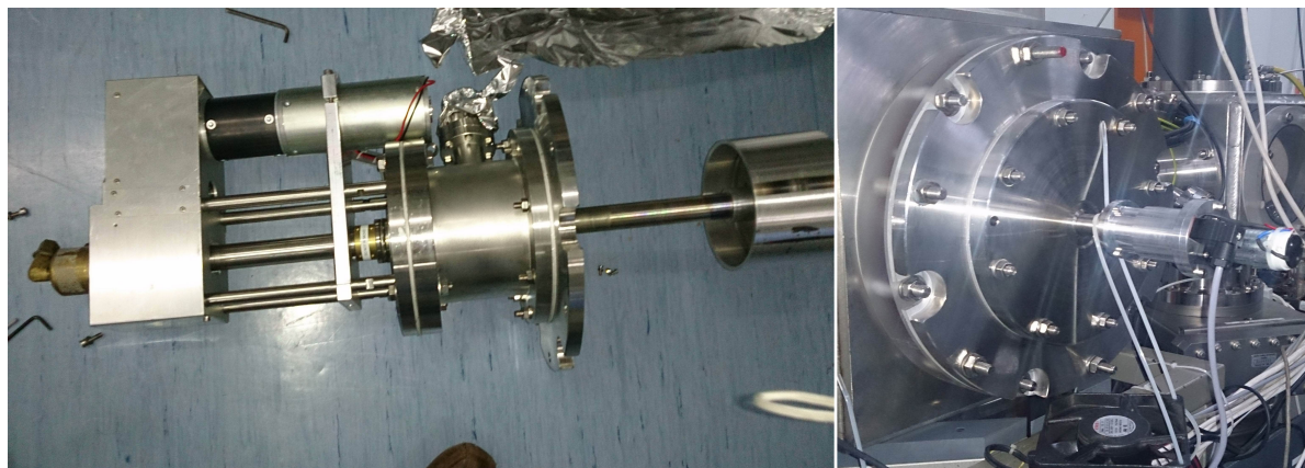
Figure 4.3.: Left panel: The dual stage reduction gear together with the massive motor of the first upgrade fixed to the outside of the chamber flange. The drive shaft connects the gear unit with the substrate passing through a rotary feedthrough. Right panel: After abandoning the water cooling of the substrate, a small motor with a single-stage reduction gear are sufficient for rotation at higher speed.
