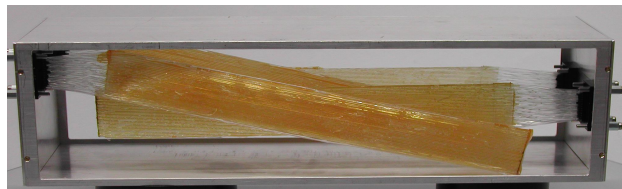
Figure 4.24: Holding frame with mounted SFT modules, side walls removed. For final operation, side open side walls are covered by light-tight black tape.
