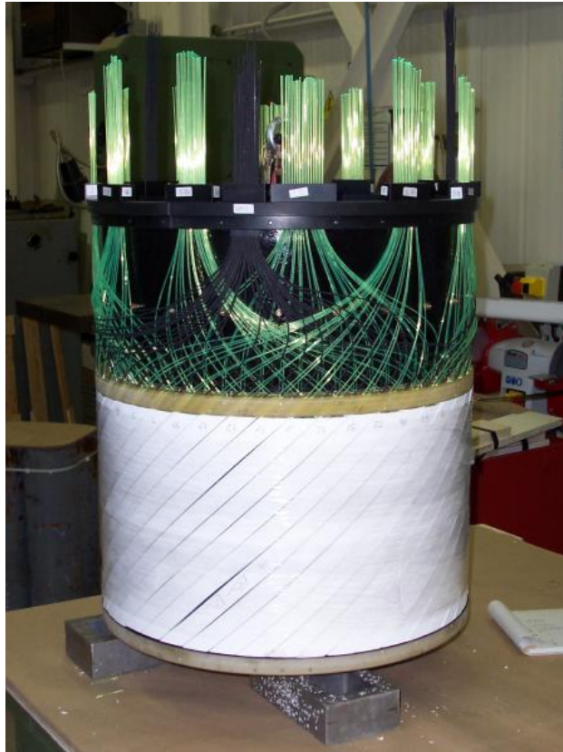
Figure 3.8: Assembling of the Photon Detector. The light tight supporting shell is missing. The scintillator strips of outer stereo layer and wavelength shifting fibres are visible. The picture was taken before the fibres have been cut at the connectors seen in the upper part of the picture.
