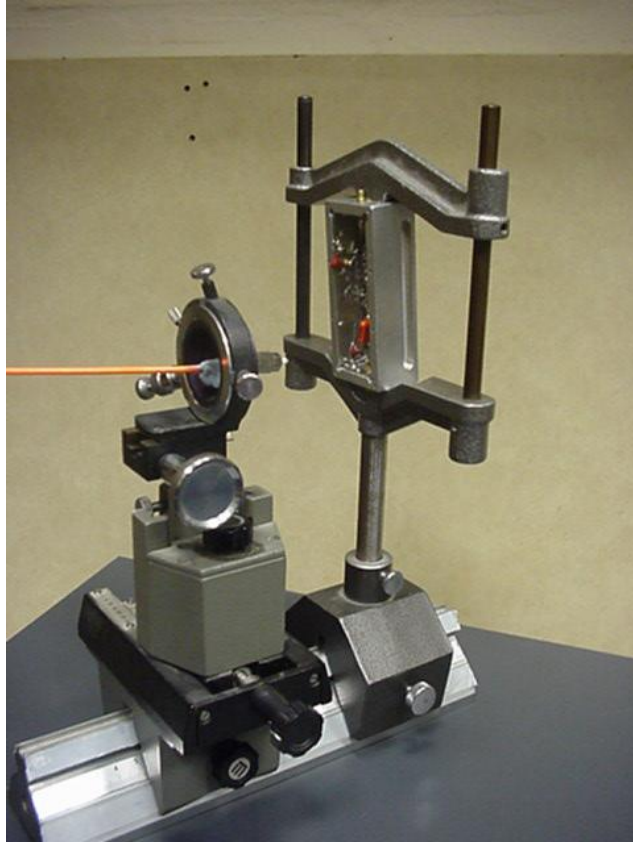
Photos K: Position of Optical Transmitter and Receiver
