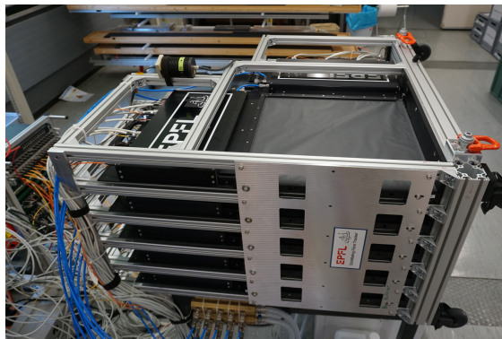
Figure 11: The SciFi tracker detector setup in the lab for cosmic ray test. The active area of a tracker module is 40\text{ cm} \times 40\text{ cm} and consists of 5 xy fibre planes.
