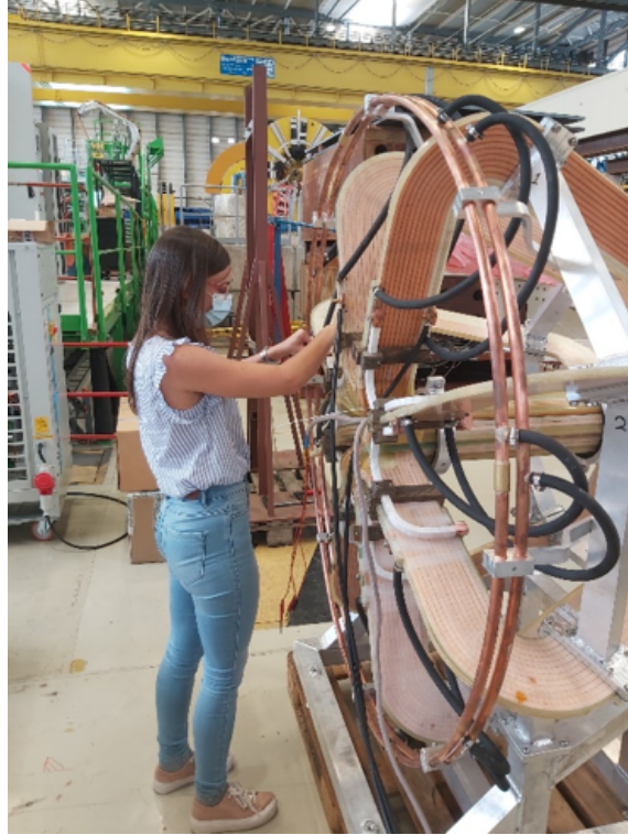
Fig. 67: Step-by-step measurement of coil, busbar, and joint resistances.
